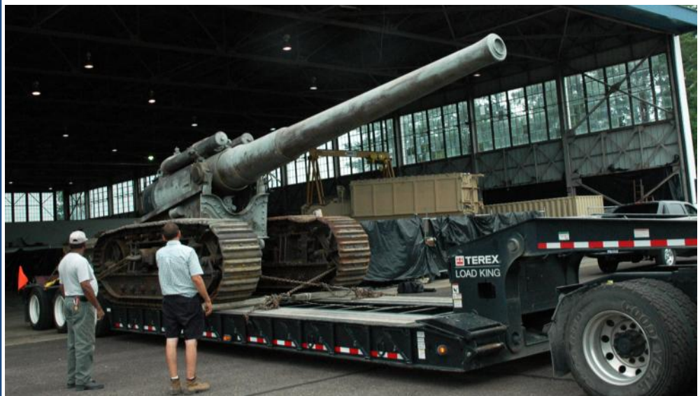
Dahlgren personnel prepare to off-load a World War I-era tractor-mounted artillery piece, the first gun test-fired at Dahlgren (then called Naval Proving Grounds Lower Station) on October 16, 1918. The 7-inch, 45 caliber gun will be restored by the Naval Surface Warfare Center Dahlgren Division. U.S. Navy photo, July 20, 2009
